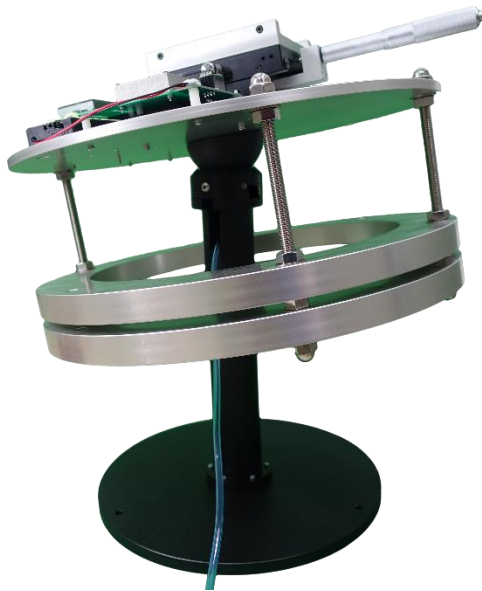
Figure 9: The air-bearing platform.
